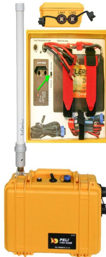
Figure 1: Outdoor resistant WLAN box. Hardware components: RaspberryPI, battery pack, Bullet M2.
