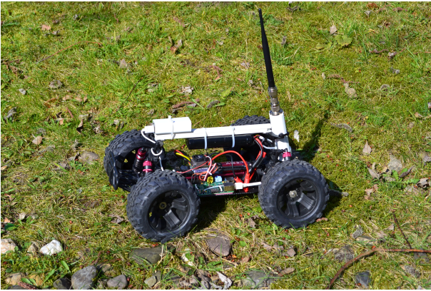
Figure 3: The Fast Mover. Attached components: RaspberryPI, battery pack, Bullet2M Router. A video with an attached network camera can be found at: http://www.youtube.com/watch?v=qVALTltiF6o
