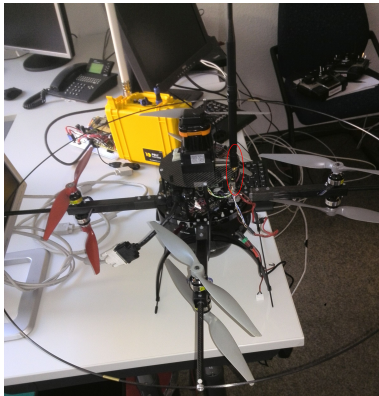
Figure 5: First test scenario: UAV with a bullet connected via WLAN to the netserver box.
