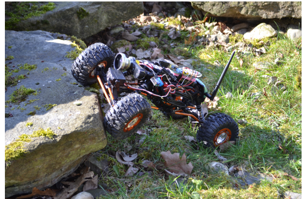
Figure 2: The Rock Crawler in action. Attached components: RaspberryPI, battery pack, ALFA WLAN Adapter and a wide angle Logitech webcam with a microphone. A video can be found at: http://www.youtube.com/watch?v=St8QtC1kut0 .
