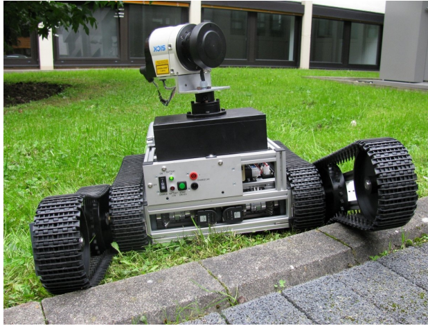
Fig. 1. The new RescueBot robotic platform with a small and robust 3D Laser range finder.
