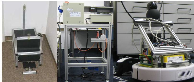
Fig. 4. Docking stations for the automatic battery charging. Left: VolksBot, Middle: Handycart. The arm is moving out if the robot it detected via infrared light, Right: The Roomba has an additional battery pack for the laser scanner and a digital relay card to switch power to the notebook if necessary.
