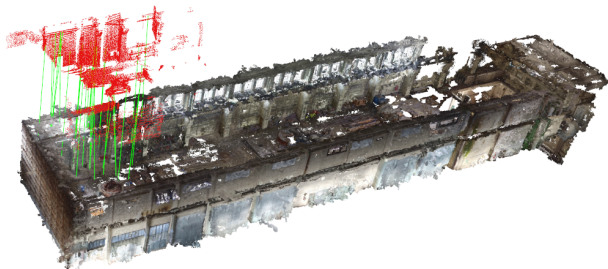
Fig. 5: Resulting global localization between 3D UGV sub-map (red point-cloud) and global 3D UAV map (coloured point-cloud). Green lines indicate the resulting descriptor matches associated to points in the two point-clouds. The data stems from the Dortmund indoor dataset and drawn from the complex experimental set-up.
